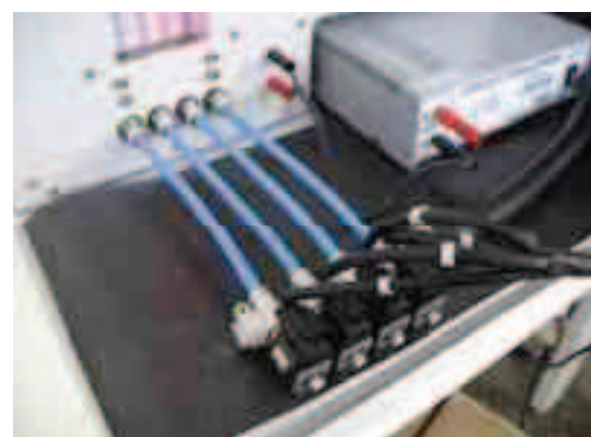
Fig. 3. Measuring device used to measure the flow rate of injectors
