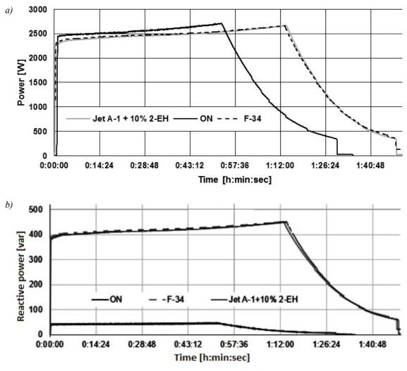
Fig. 3. Battery charging process: a) active power of generator powered with Diesel (black line)
