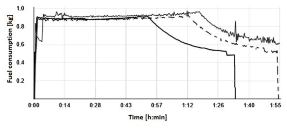
*Fig. 2. Power generator momentary fuel consumption (kg/h) for three different fuels: Diesel (black) F-34 (black dashed) and Jet A-1 (grey)*
