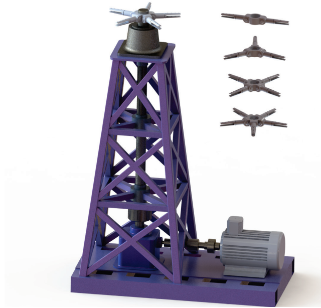
Fig. 6. Concept of the whirl tower system with horizontally mounted engine
