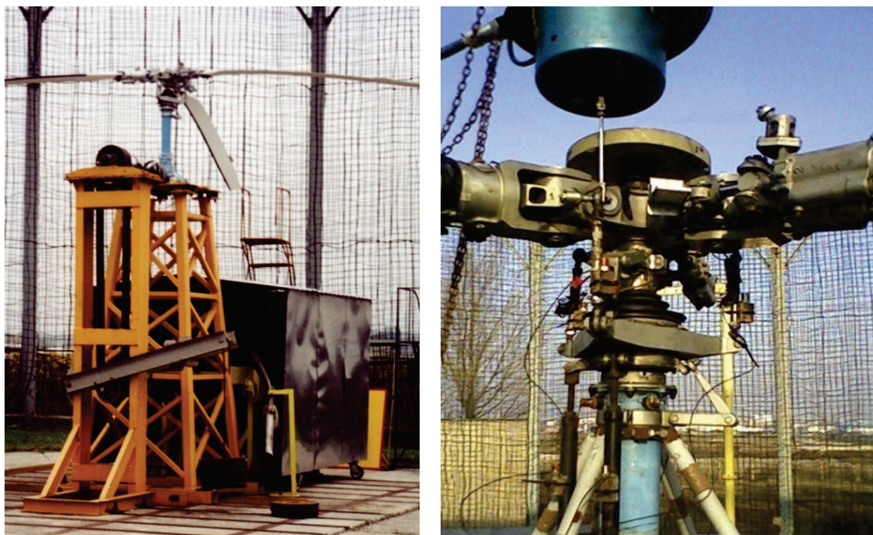
Fig. 4. The whirl tower system for helicopter three-blade main rotor
