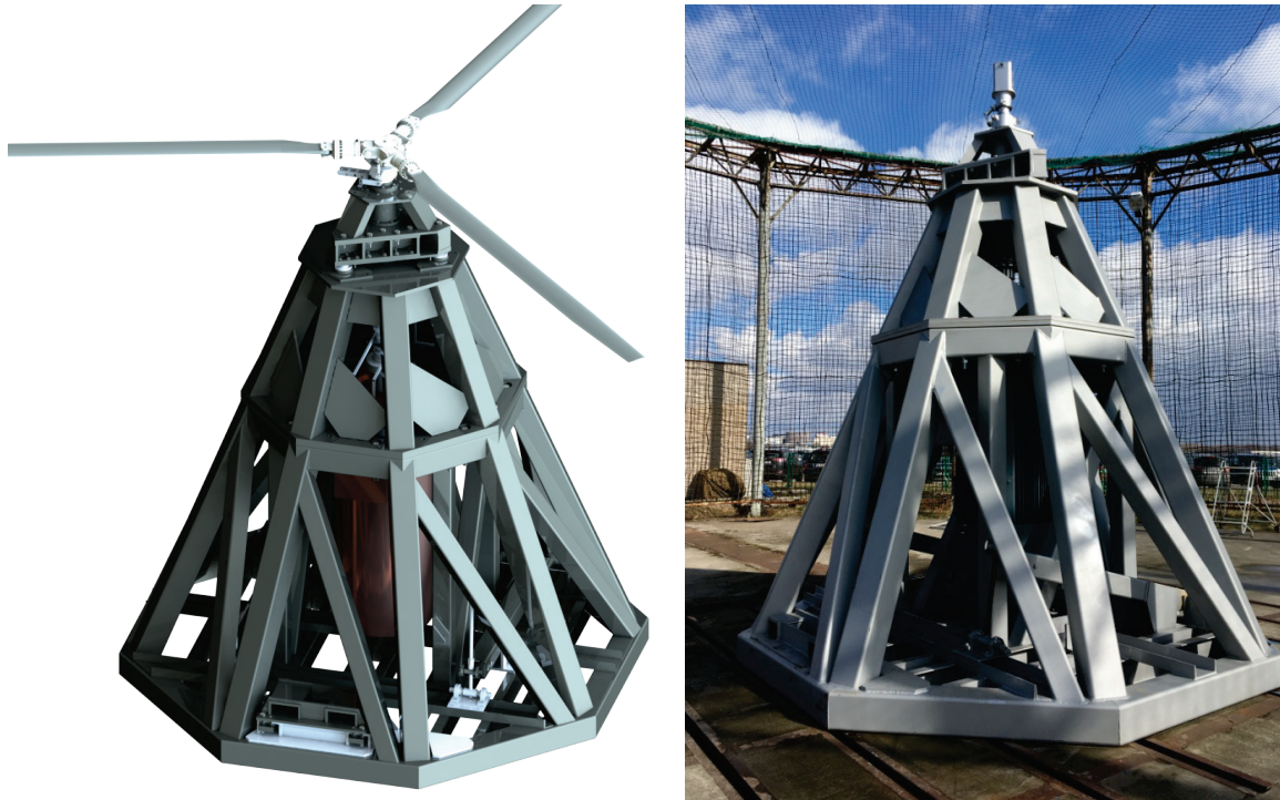
Fig. 8. New whirl tower: visualization with rotor hub and blades (left), frame of the whirl tower with the mounted engine (right)
