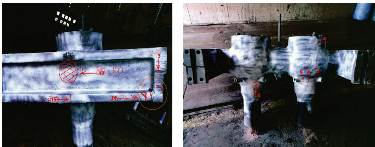
Fig. 1. Detected material discontinuities, magnetic-powder testing
