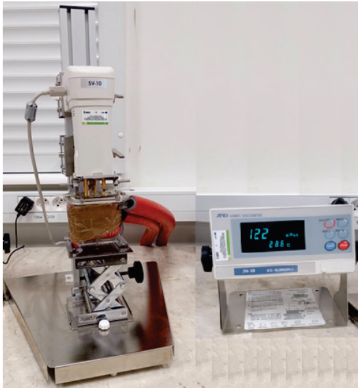
Fig. 4. Measuring stand: a) vibratory viscometer SV with vibrating fork, b) water jacket, c) sensor unit [17]
