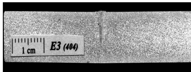
Fig. 3. The melting depth approximately 8 mm. The face is 3.5 mm wide.; there are two little ball-like air sacs \phi 0.2 mm (2011) pursuant to PN-EN 30042:1994
