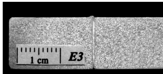
Fig. 1. AlMg3 alloy melting with electron beam through the sheet; the face of the weld is concave, up to 2.2 mm wide; narrow weld of equal width; the root effluent all over the melting length
