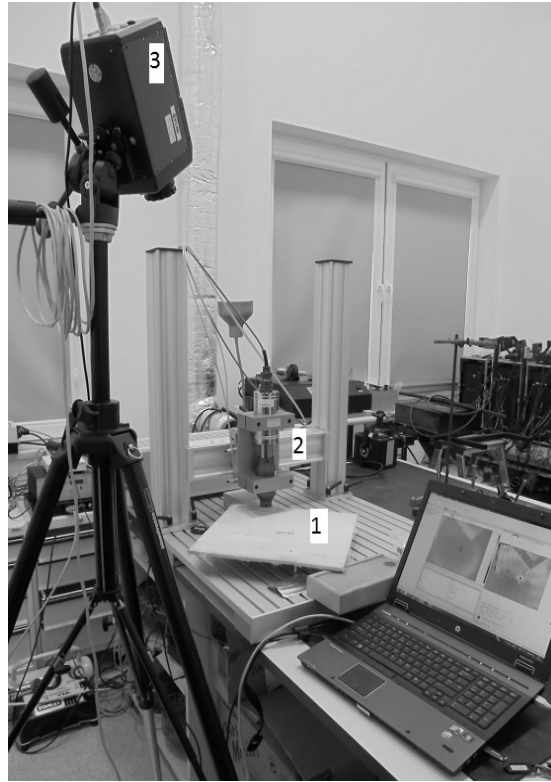
Fig. 1. The test stand: 1 – sample, 2 – ultrasonic source, 3 – thermal camera
