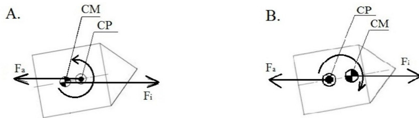
Fig. 4. Projectile shape according to PN-EN 15152:2007 – force distribution: A – unstable, B – stable; where: CM – centre of mass, CP – centre of aerodynamic pressure, F_a – aerodynamic force, F_i – inertia force
