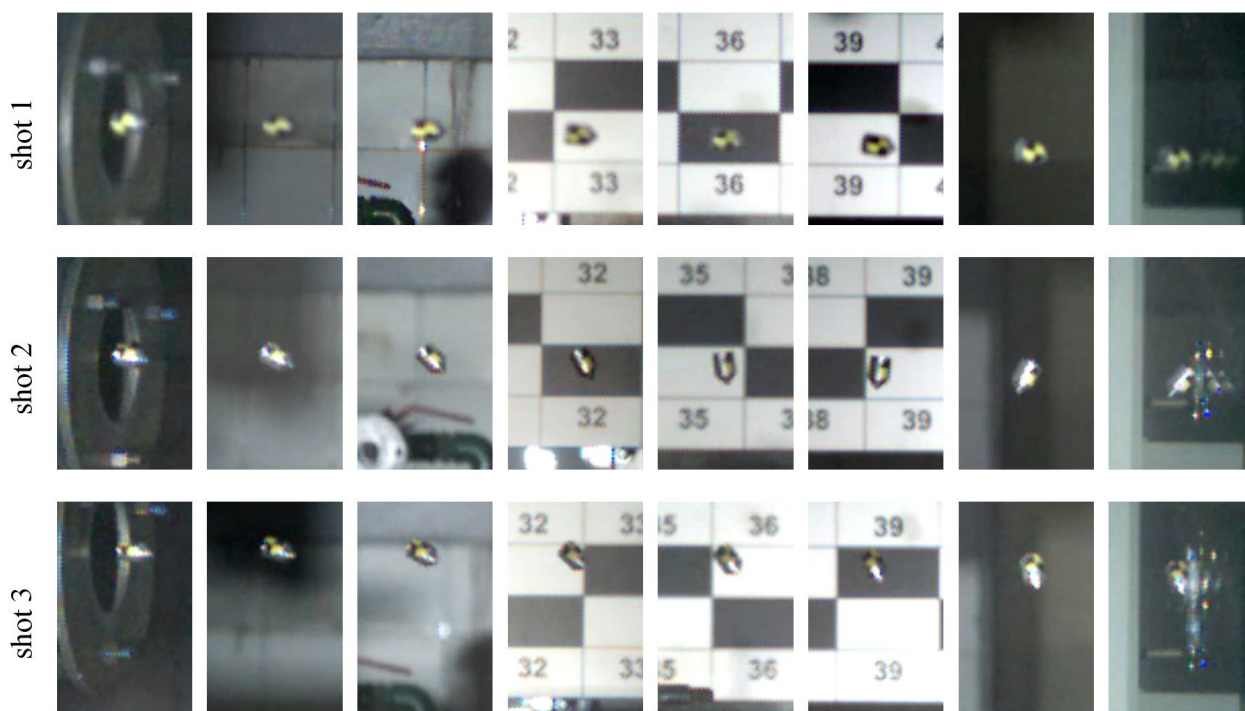
Fig. 1. Trajectory of projectile, performed in accordance with the standard guidelines [6], during 3 impact tests recorded with a high-speed camera
