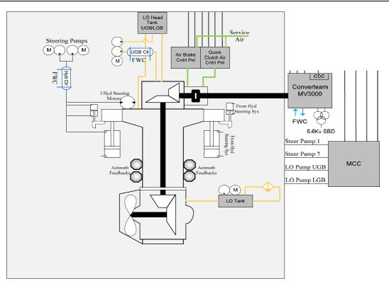
Fig. 2. An arrangement of azimuth thruster auxiliary system [1, 5]
