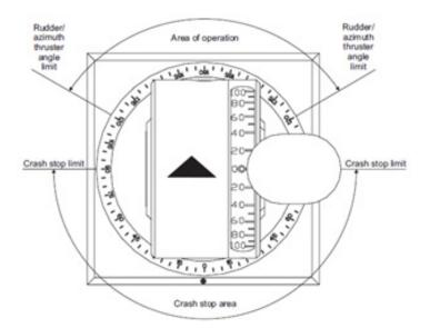
Fig. 7. The limitations of thruster angle rotation (area of operation) or thrust limits [1]
