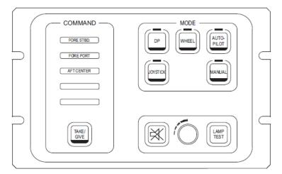
Fig. 4. The main operating modes of propulsion system steering – steering panel [1]
