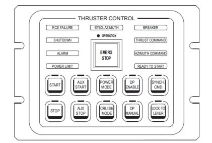
Fig. 5. Thruster Control Panel [1]
