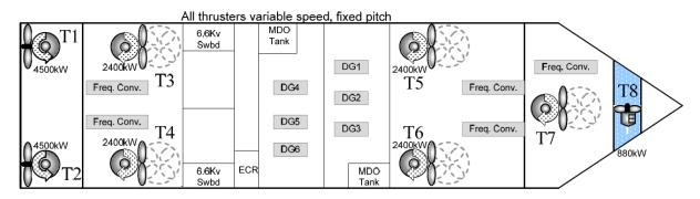
Fig. 1. Propulsion system of a pipe-layer vessel mv Global 1200 [1]
