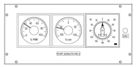
*Fig. 6. The essential work indicators of a thruster: from left side: the percentage of nominal power indicator, the percentage of nominal speed, the direction of thrust in comparison to main vessel axis [1]*
