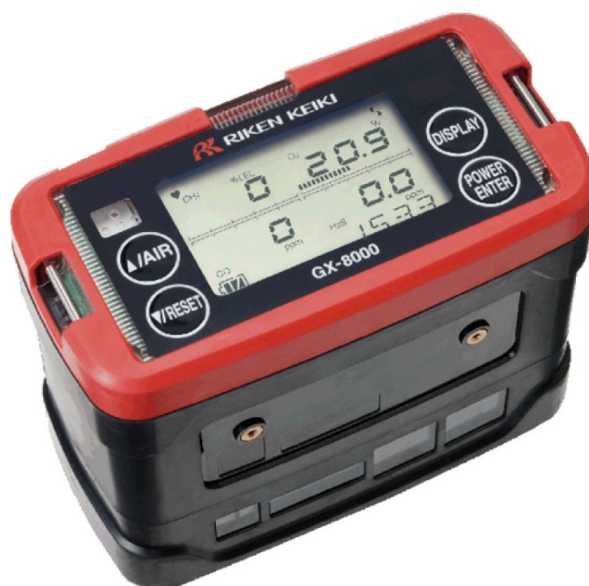
Fig. 7. Portable gas detector Riken Keiki GX-8000
