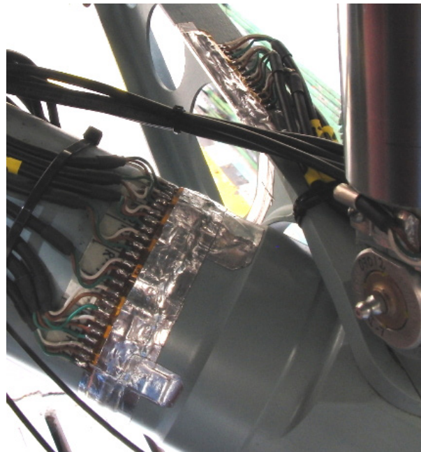
Fig. 2. Strain gauges mounted on the landing gear (example) [source ILot]
