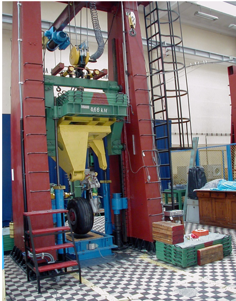
Fig. 4. Free fall dynamic drop test machine example. Note the ground plate below the landing gear [source ILOt]
