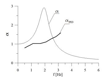
Fig. 8. Frequency response of passive and active systems
