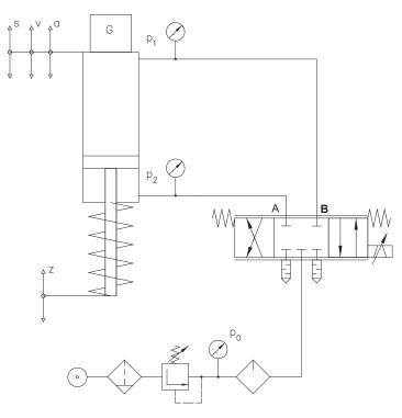
Fig. 3. Schematic diagram of control of the pneumatic cylinder
