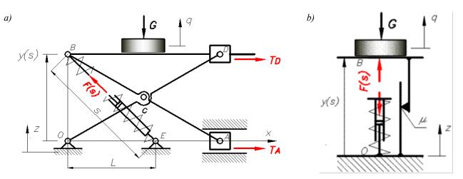
Fig. 1. Kinematic system of the seat suspension (a). Replacement model of the active seat suspension (b)
