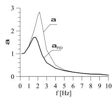
Fig. 2. Transmissibility function of a regulated single-acting pneumatic actuator
