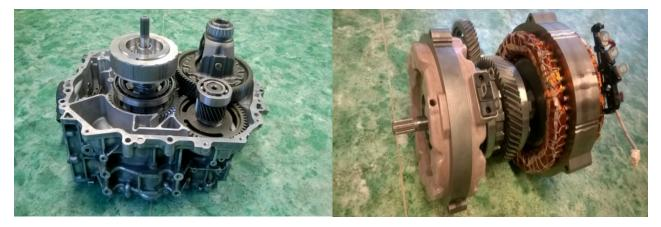
Fig. 2. Electronically controlled continuously variable transmission (eCVT)[8]
