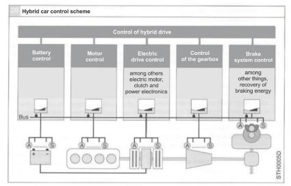
Fig. 3. Hybrid power train control system [2]
