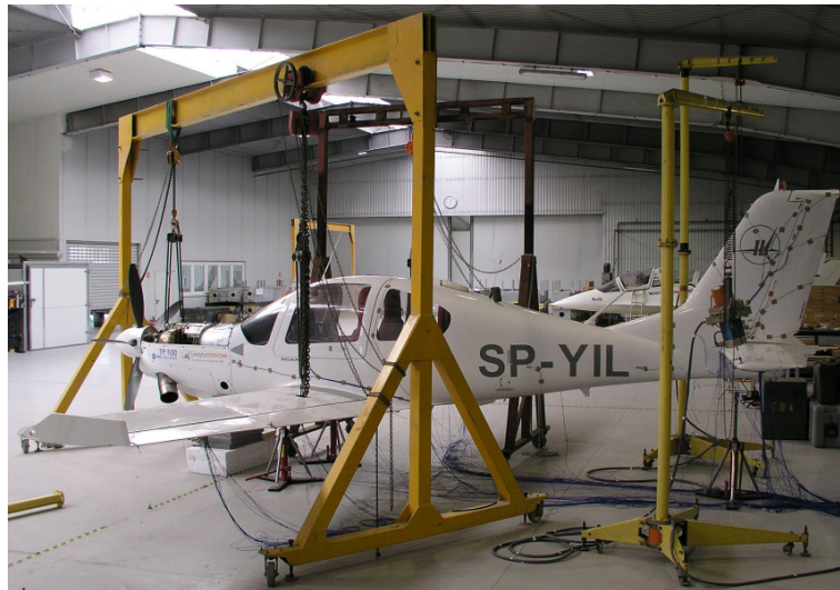
Fig. 1. GVT of the I-31T turboprop aircraft (I-23 after the power plant change), 2015
