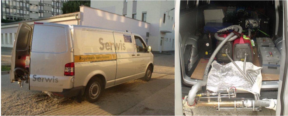
Fig. 5. Test vehicle equipped with measuring devices and additional load
