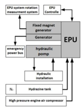
Fig. 1. A functional diagram of EPU system of emergency power supply EPS of F-16 multirole aircraft
