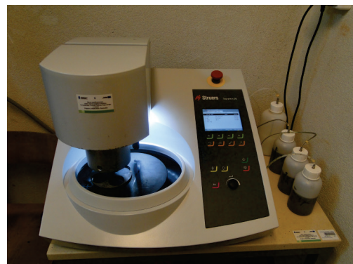
Fig. 2. The process of preparation of metallographic sections using a STRUES type Labotom 5 grinder
