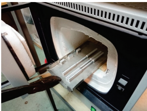
Fig. 1. The sample aging process in the SNOL furnace model 8,2 / 1100
