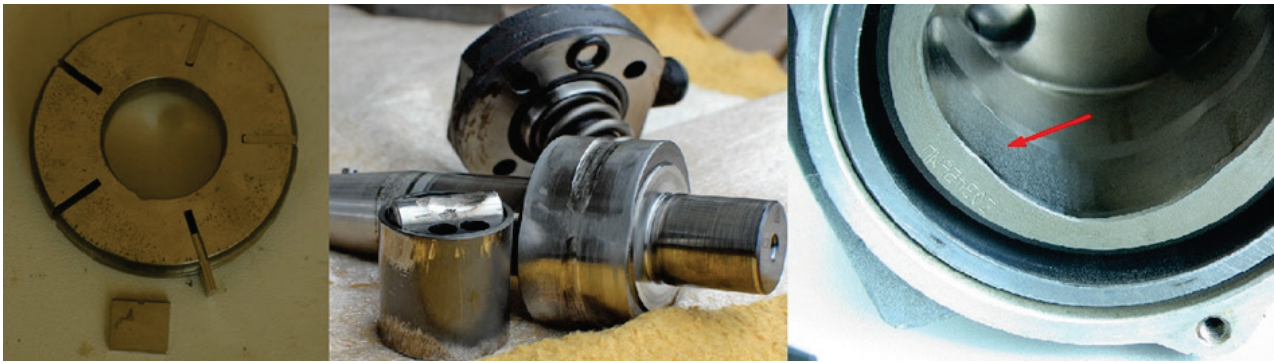
Fig. 2. Examples of damage of pumps by various producers, starting from left: Continental DHP, Bosch CP4 Delphi DFPI [3]
