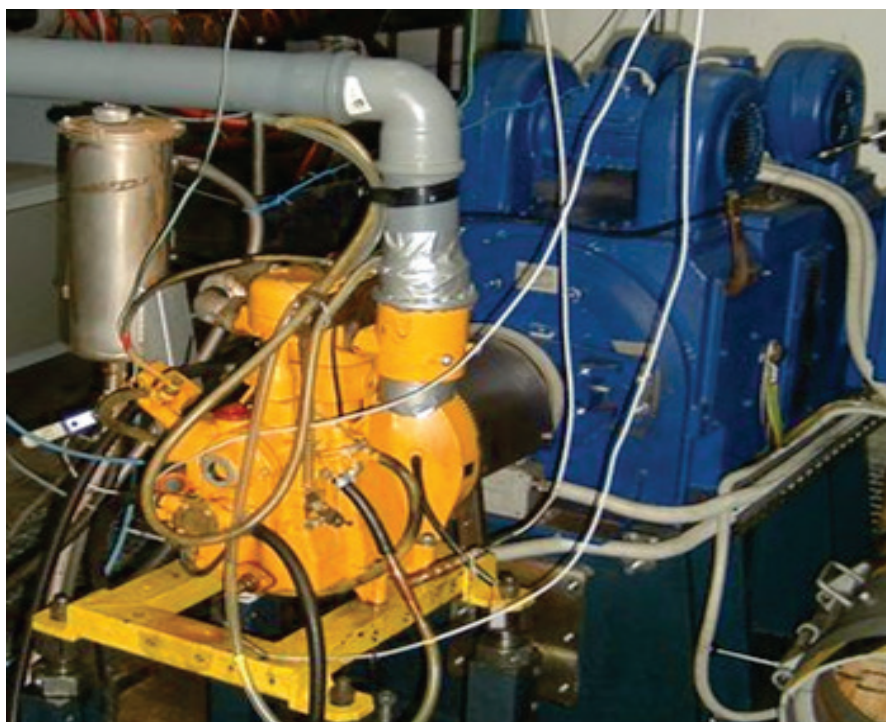
Fig. 2. Engine of 18 W type installed on test bench
