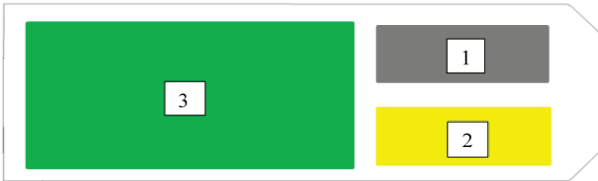
Fig. 3. Vehicle compartments: 1 – driver, 2- power unit, 3 – role-dependent
