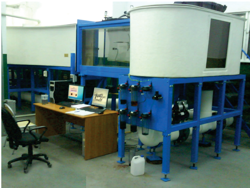
Fig. 3. Wroclaw University of Technology water tunnel (Rolling Hills Research Corp. Water Tunnel model 2436) [40]
