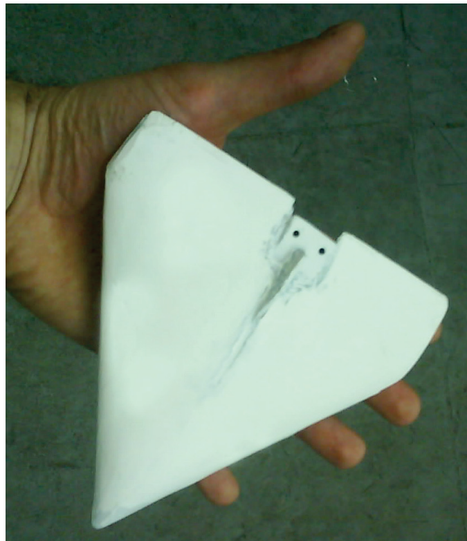
Fig. 5. Delta wing model
