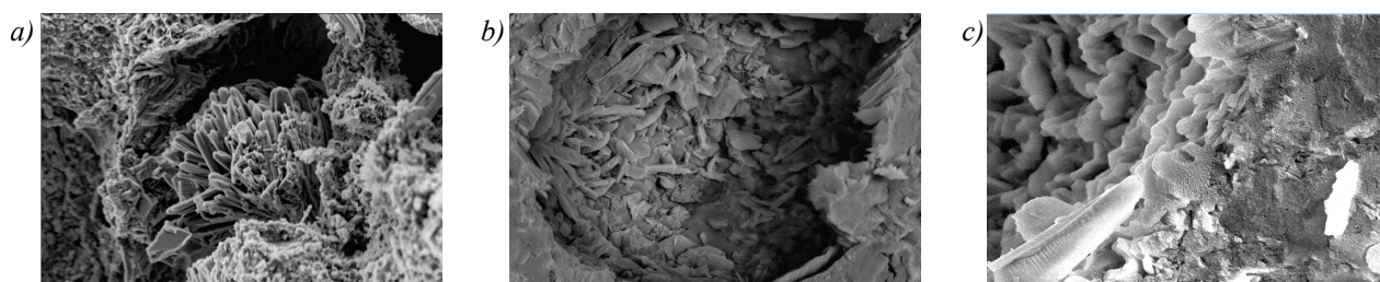
Fig. 1. Internal microstructure of selected sections (cement matrix) in concrete a) BM_{Mt} , b) \acute{s}wBM_{Mt} and c) ^{200}BM_{Mt}
