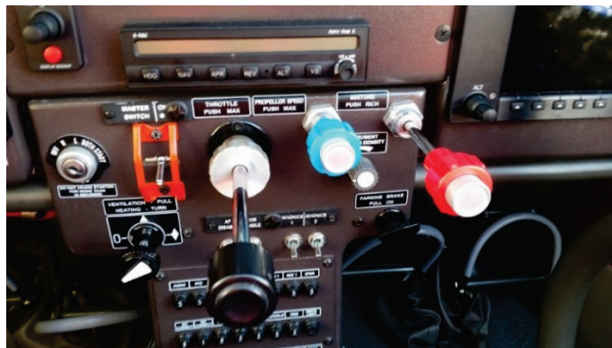
Fig. 2. Control levers of the propulsion unit in the aircraft Zlin 143LSi
