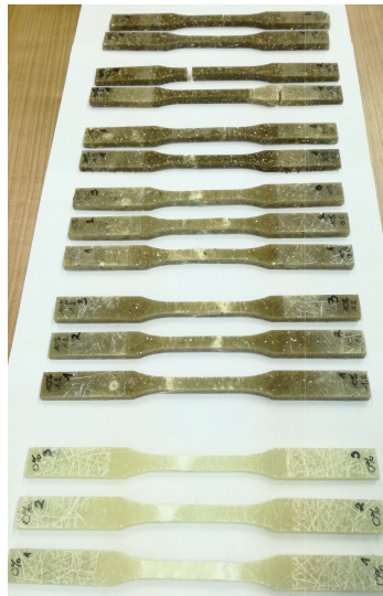
Fig. 5. Samples after static tensile testing
