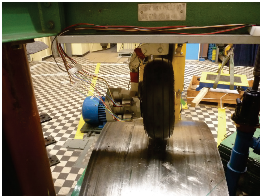
Fig. 7. Brake mounted on Mlot 3T test stand
