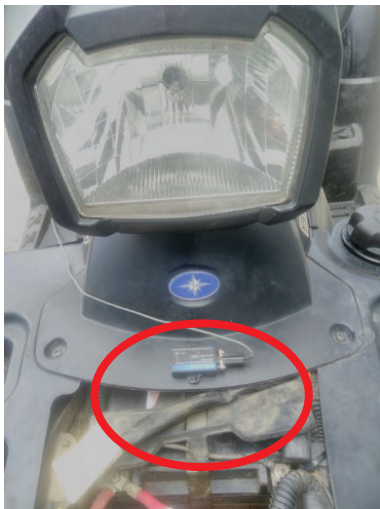
Fig. 4. Placement of the 3DM-GX3-25 sensor on the vehicle during tests
