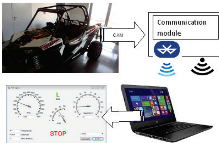
Fig. 3. A flow chart of designed data visualization system
