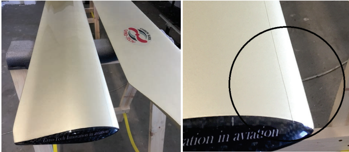
Fig. 6. Test object – blades with anti-erosion tape (0.2 mm thickness)
