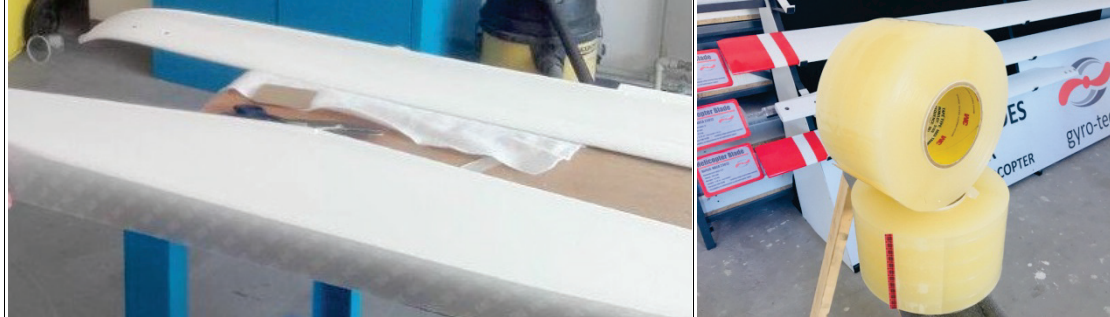
Fig. 1. Example of anti-erosion tape (Polyurethane Protective Tape) on left ILX – 27 blades coating with tape on right tape used by Gyro-Tech Company
