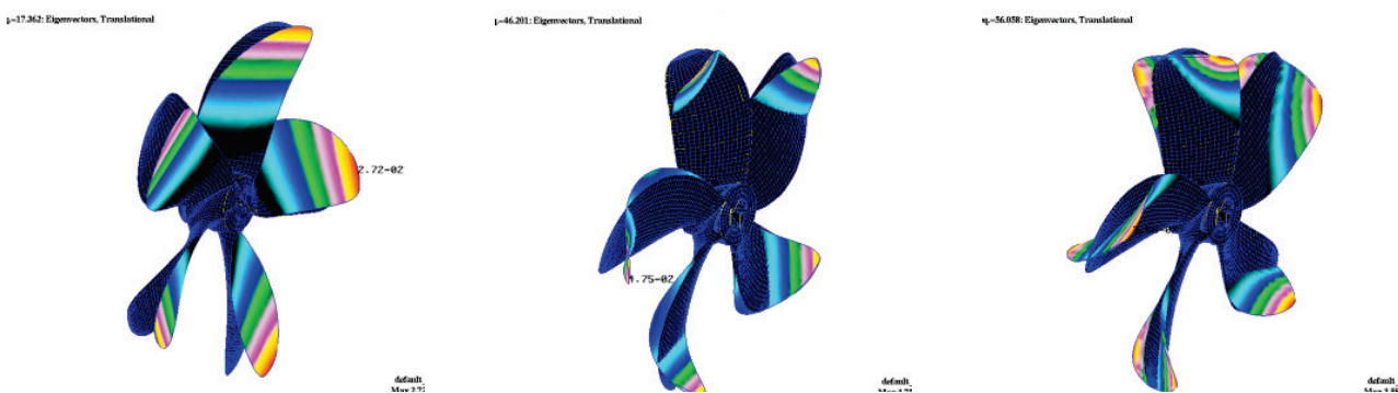
Fig. 2. First three natural modes of the propeller
