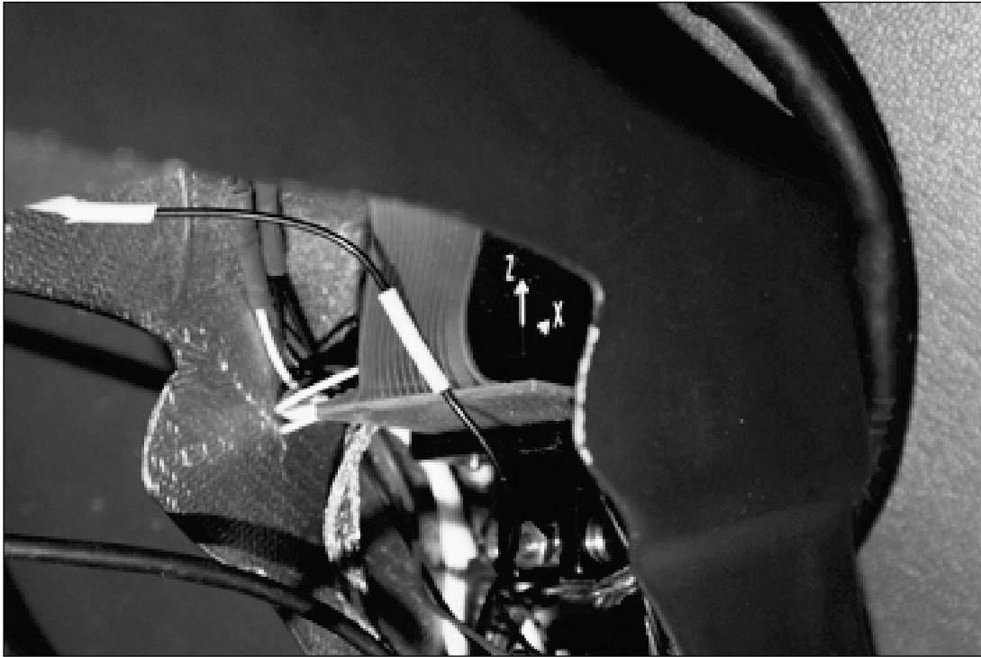
Fig. 6. A view of the integrated ADIS-16405 three-axis sensor built into the pilot's helmet [own study]
