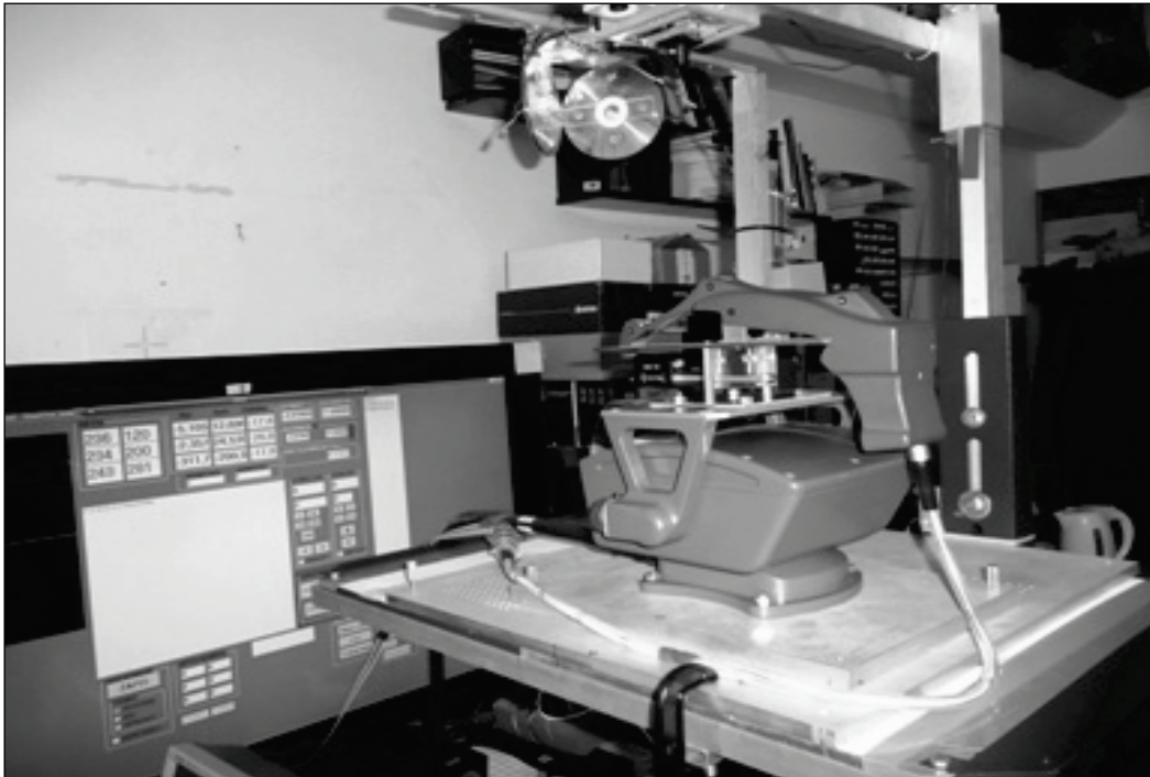
Fig. 5. A view of the integrated ADIS-16405 three-axis sensor built into the pilot's helmet during the experimental researches with magnetic field generated by the electrical flat coils [own study]
