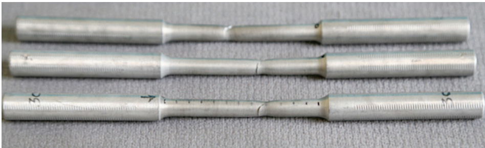
Fig. 7. Samples: 3A, 3B, 3C – artificially aged with a visible neck
