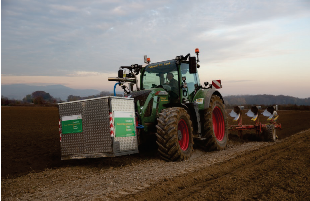
Fig. 2. PEMS measurement during ploughing with a vegetable oil compatible tractor Fendt 724 SCR (Stage IV)
