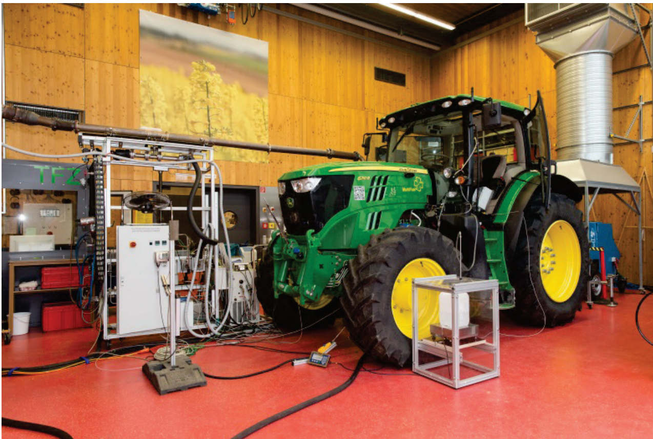
Fig. 1. Emission measurement based on legal test cycles with a John Deere 6215R (Stage IV) at the tractor test stand
