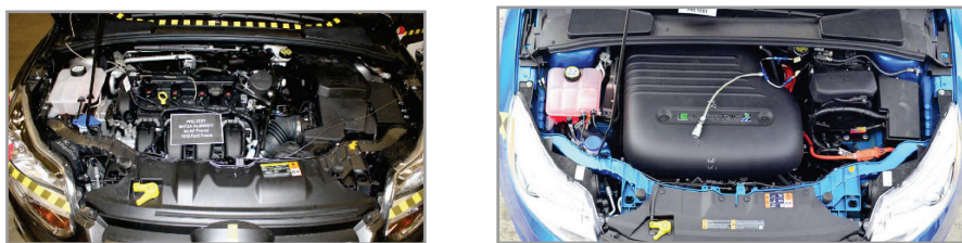
Fig. 8. Ford Focus car silhouettes – ICE on the left, BEV on the right [12]
