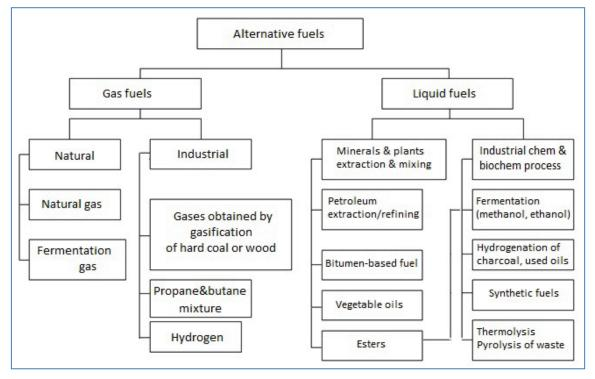
Fig. 3. Types of alternative fuels used in combustion engines (based on [3])
