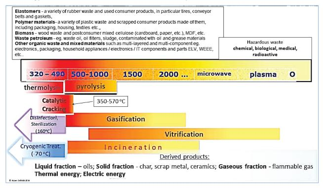
Fig. 5. Methods of thermal treatment of organic and mixed waste [2]
