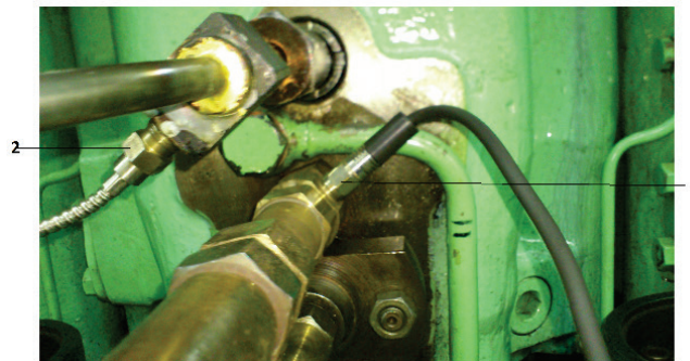
Fig. 6. The research stand with the marine diesel engine Sulzer 3AL25/30 – view on one of cylinder heads of the mounted sensors: 1 – injection press sensor Oprand AutoPSI-S, 2 – combustion press sensor Kistler 6353A24
