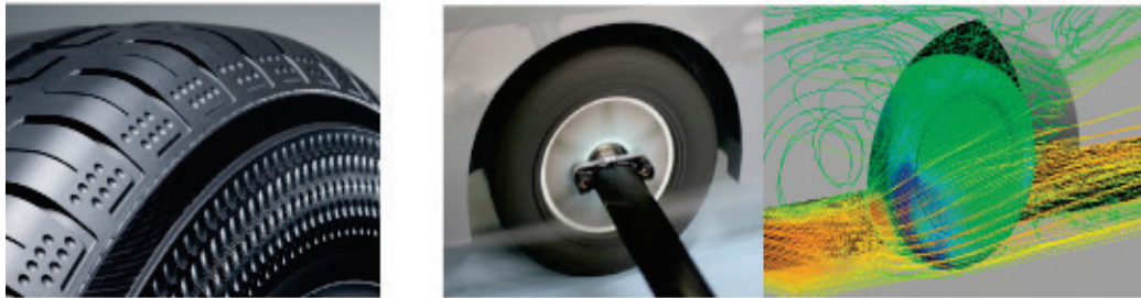
Fig. 18. Dimpled design reduces air resistance (left) and data gleaned from wind-tunnel simulations helped to optimize tyre shape – tread and dimple configuration (right) [18]
