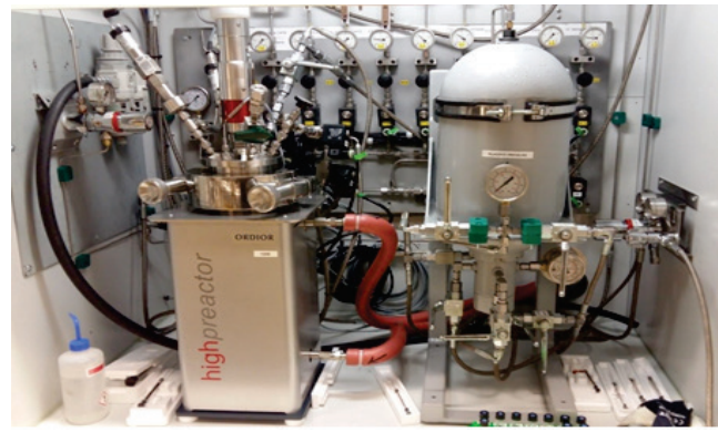
Fig. 1. Mixing reactor of methane and propane fuels
