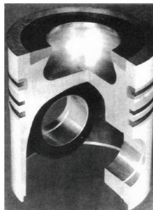
Fig. 2. Piston made by Toyota Inc. with the metallic composite inserts [12]
