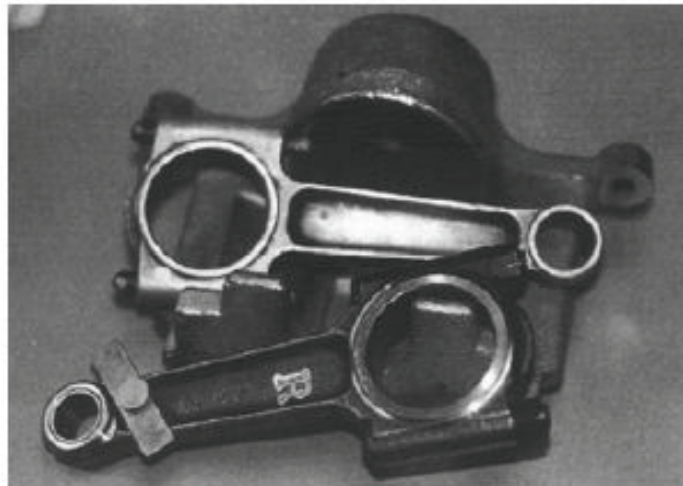
Fig. 4. Connecting rods of metal composite [12]
