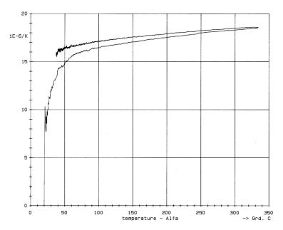
Fig. 1. Thermal expansion coefficient as a function of temperature from ambient temperature to 350°C during heating and cooling of the novel composite alloy
