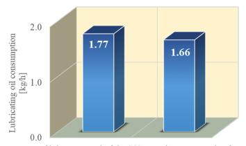
Fig. 8. Hourly consumption of lubricating oil of the S12-U with pistons made of novel composite alloy
