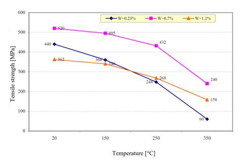
Fig. 3. The relationship of tensile strength in the temperature function of alloys containing different amount of tungsten
