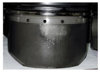
Fig. 11. Friction markers formed on a piston surface which appear during engine operation
