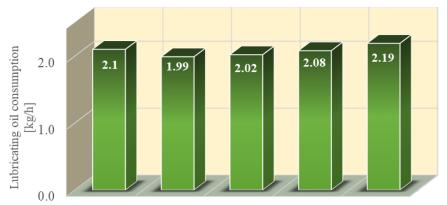
Fig. 9. Hourly consumption of lubricating oil of the S12-U with pistons made of novel composite alloy PA alloy of forget piston
