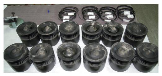
Fig. 10. View of the novel composite alloy pistons after engine testing
