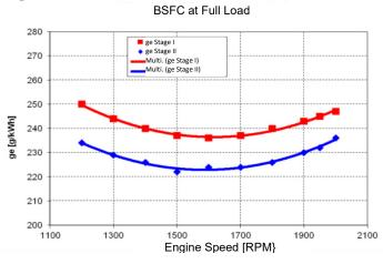
Fig. 6. Comparison of specific fuel consumption (BSFC) as an engine speed function of the tested S12-U engine with pistons made of novel composite alloy and PA alloy forged pistons at full load operation
