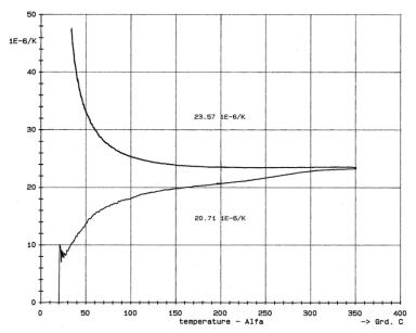
Fig. 2. Thermal expansion coefficient as a function of temperature from ambient temperature to 350°C during heating and cooling of the forged piston PA alloy
