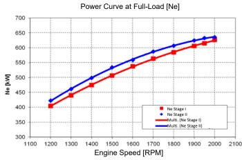
Fig. 5. Comparison of the S12-U power with pistons made of novel composite alloy and PA alloy forged piston
