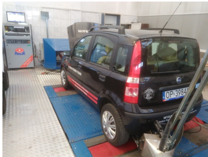
Fig. 1. Test object and chassis dynamometer test stand
