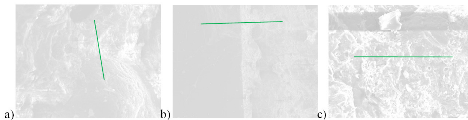
Fig. 3. Exemplary microanalysis of BM concrete: a) contact area between fine aggregate grains and cement matrix, b) contact area between coarse aggregate grains and cement matrix, c) cement matrix
