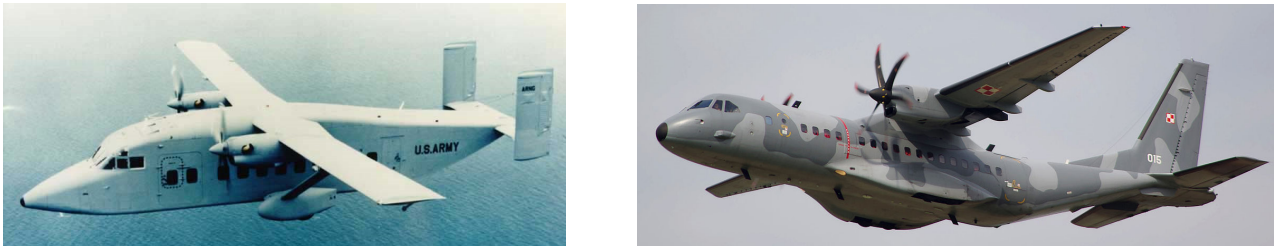
Fig. 1. Examples of present multi-engine airplanes in which the propeller slipstream and aerodynamic wake behind the propulsion unit can affect the operation of the tail assembly, Shorts C-23 Sherpa (left), CASA C-295 (right) [4, 3]
