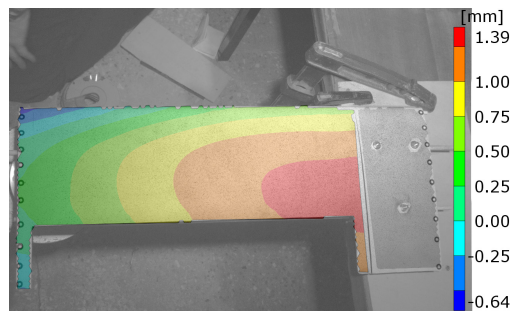
Fig. 8. Example of ARAMIS system measurement result – displacement along the wingspan
