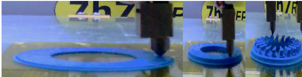
Fig. 1. Example of a model being made with FFF
