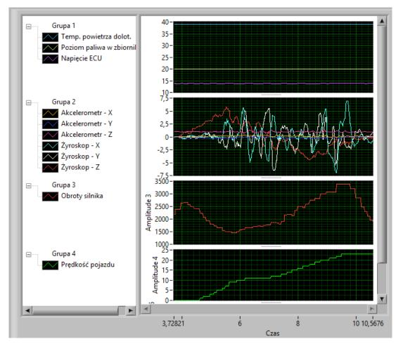
Fig. 4. The example of monitored parameters in road test
