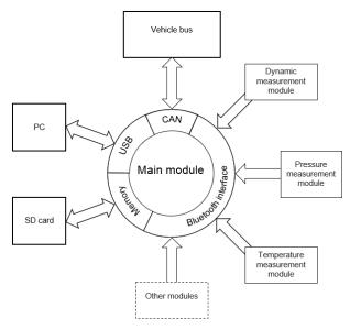
Fig. 1. The conception of modular monitor of car exploitation parameters in motion
