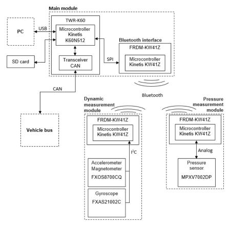
Fig. 2. The scheme of the prototype of modular monitor of car exploitation parameters in motion
