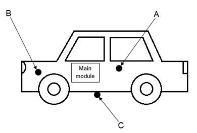
Fig. 6. The location sensor modules during the communication test (A - passenger compartment, B - engine compartment, C - under the chassis)
