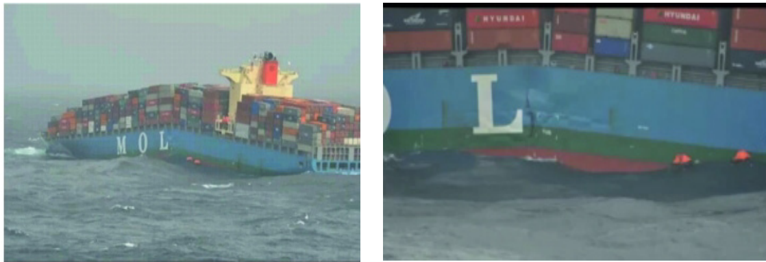
Fig. 1. Container ship fracture as a result of severe weather conditions
