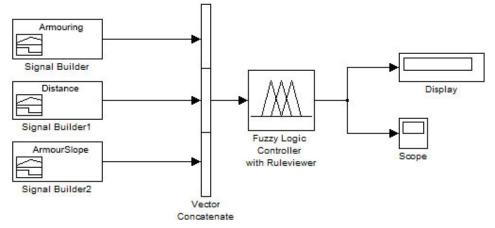
Fig. 4. Model of the designed system in Toolbox Simulink
