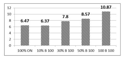
Fig. 3. Dependence of viscosity on biocomponent content
