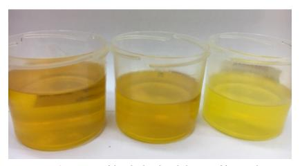
Fig. 1. Mixtures of diesel oil and methyl esters of fatty acids
