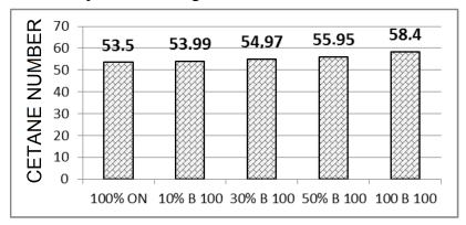
Fig. 4. Mean values of cetane number for variable contents of a biocomponent in a fuel
