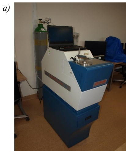
Fig. 3. a) Solaris-ccd plus optical spectrometer b) the sample used for the chemical composition testing
