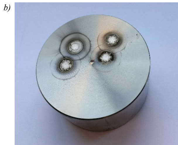
Fig. 3. a) Solaris-ccd plus optical spectrometer b) the sample used for the chemical composition testing
