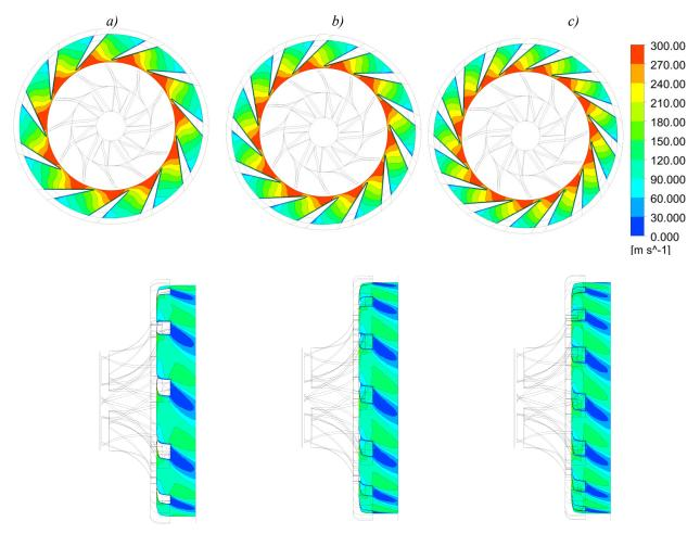
Fig. 6. Velocity distribution in diffuser area a) 11 blades, b) 13 blades, c) 15 blades
