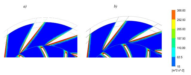
Fig. 3. Vanless diffuser space effect on turbulence intensity, a) value of  $x_3$  coefficient 1.0475, b) value of  $x_3$  coefficient 1.0745
