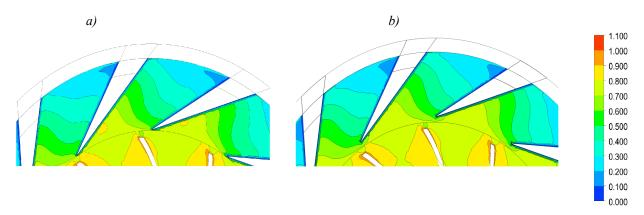
Fig. 2. Vanless diffuser space effect on a Mach number. a) Value of x<sub>3</sub> coefficient 1.0475, b) value of x<sub>3</sub> coefficient 1.0745
