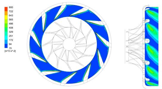
*Fig.* 10. *Modified design – turbulence intensity.*
