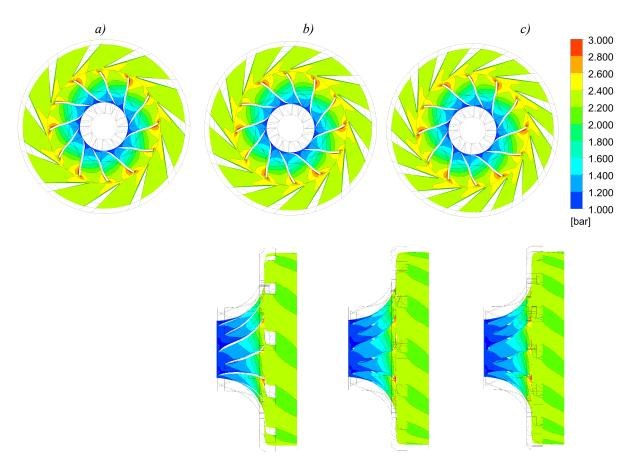
Fig. 5. Total pressure distribution a) 11 blades, b) 13 blades, c) 15 blades
