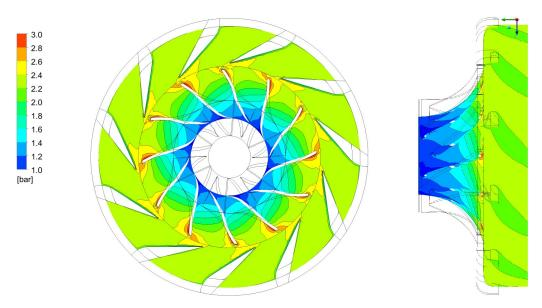
Fig. 8. Total pressure distribution in modified design
