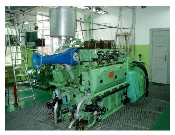
Fig. 1. Photo of the piston engine SULZER 3AL25/30
