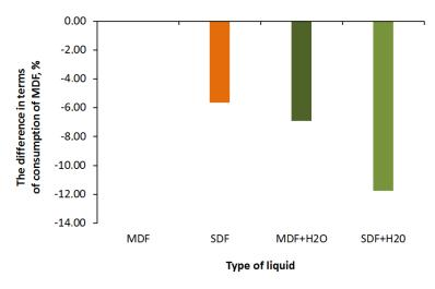
Fig. 2. Difference in fuel consumption with respect to mineral oil consumption
