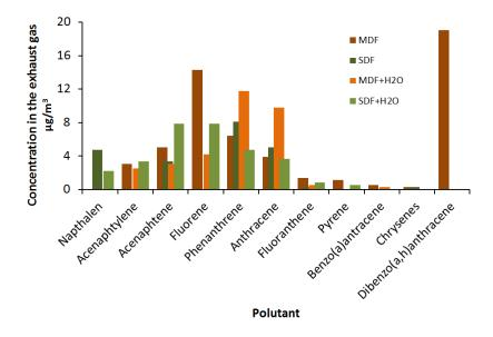
Fig. 3. Illustration of concentrations of emitted aromatic hydrocarbons (PAH) when engine is fuelled by different fuels
